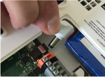
Plug in the power connector
