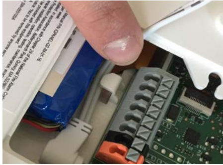
Route the wire behind the retainer clip
