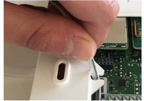
Insert the wire into the strain-relief
