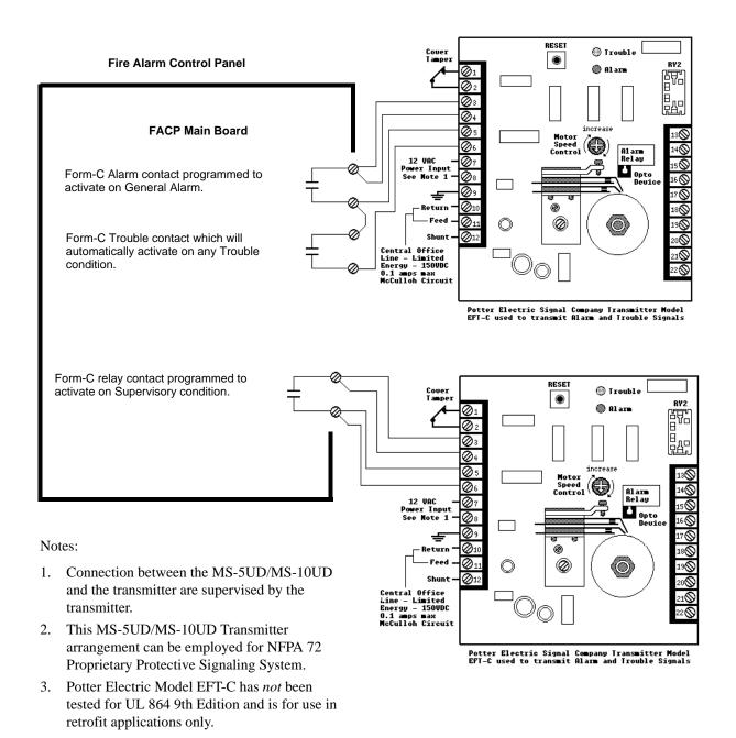
Figure B.4 Proprietary Protective Signaling System
