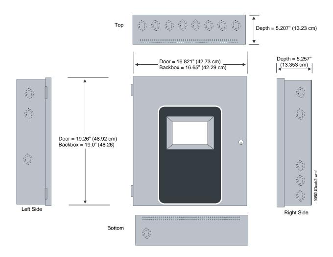
Figure 2.3 Backbox and Battery Box
