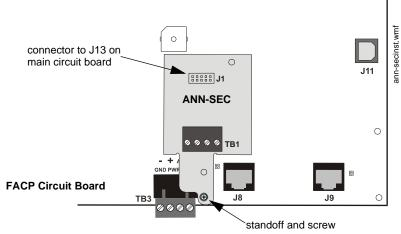
Figure 2.18 Installing the ANN-SEC Option Card
