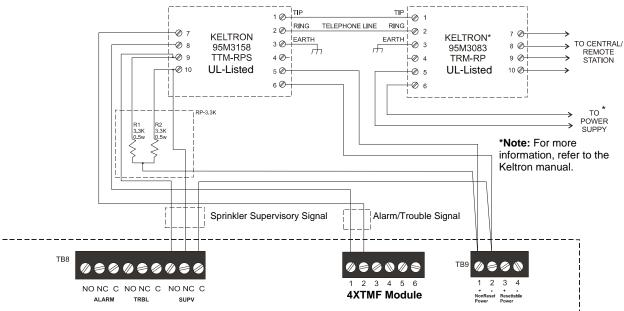
**Note:** Cut TBL jumper on 4XTMF module to send alarm/trouble signal from the same pair or terminals.
