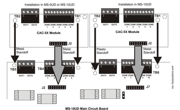
Figure 2.14 CAC-5X Module Installation
