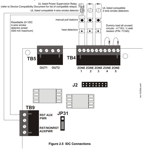
Input Circuits Installation
