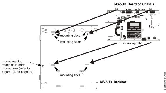
Figure 2.1 Chassis Mounting in Backbox
