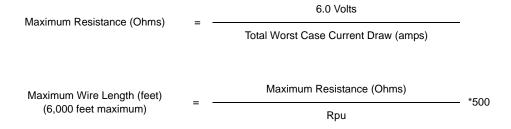
where: Rpu = Ohms per 1,000 feet for various Wire Gauges (see table below)
