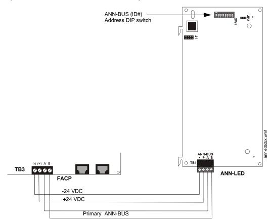
Figure 2.27 ANN-LED Board Layout and Connection to FACP
