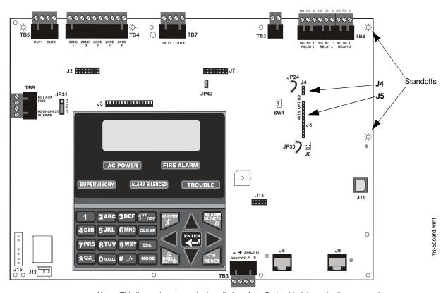
**Note:** This illustration shows the installation of the Option Module on the 5-zone panel. The module is installed in the same location on the 10-zone panel.
