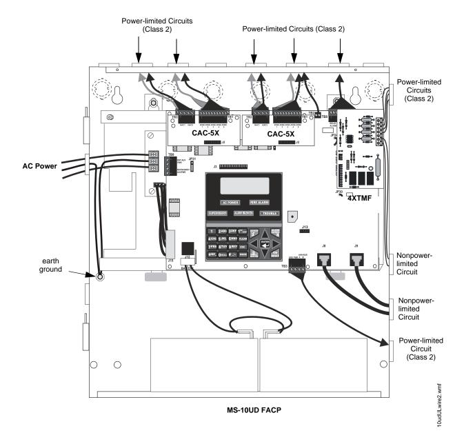
Figure 2.11 Typical UL Power-limited Wiring Requirements
