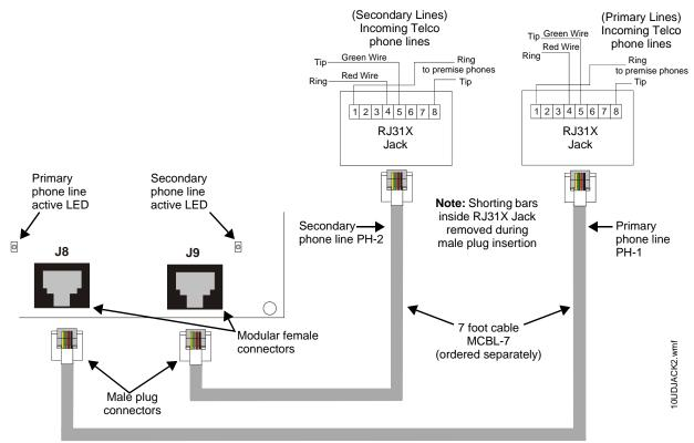
Figure 2.13 Wiring Phone Jacks
