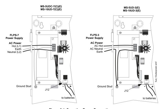
Figure 2.4 Operating Power Connections
