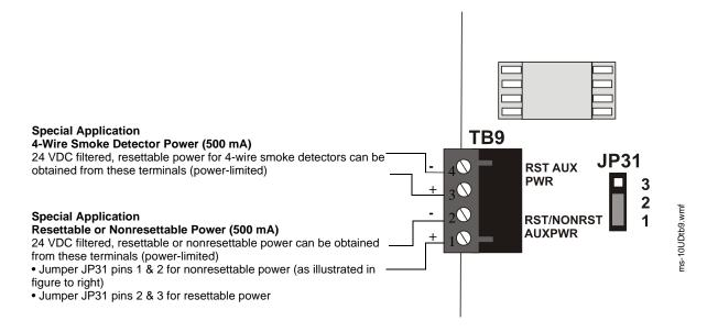
Figure 2.8 Special Application Auxiliary Power
