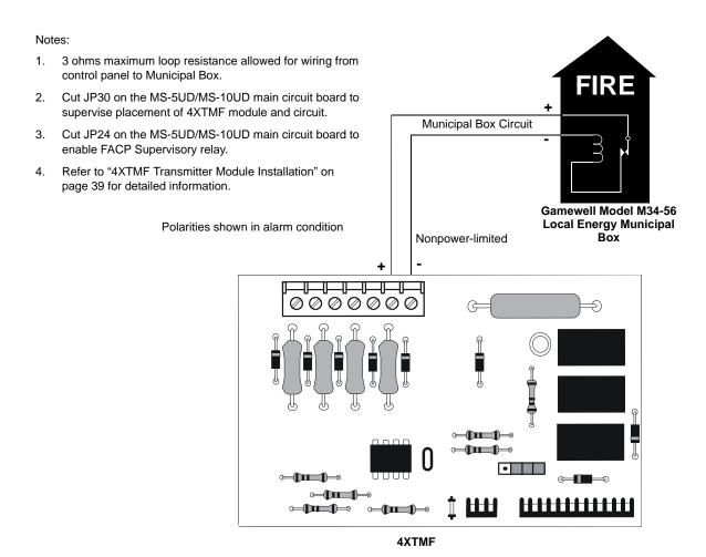
Figure B.2 Municipal Box Connected to 4XTMF Transmitter Module
