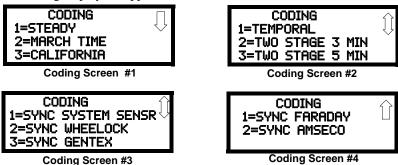
The programmer can select the notification appliance output by pressing the number corresponding to the desired output. The coding selections are:
