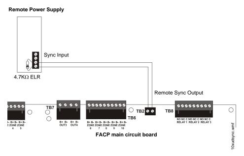
Figure 2.10 Remote Sync Output
