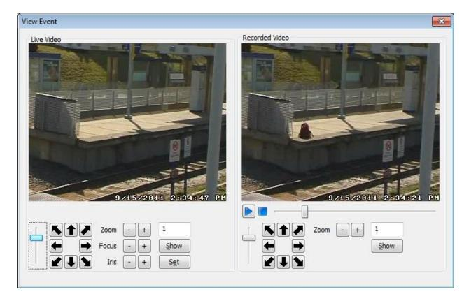
**Note:** For PTZ to operate a fixed camera in the Live Video window, the camera must be configured as a PTZ camera using the 'Digital' protocol (please reference the *Administrator's Manual* for setup instructions). Digital PTZ controls will function for recorded video on any camera, even if the camera is not configured as a PTZ camera using the 'Digital' protocol.
